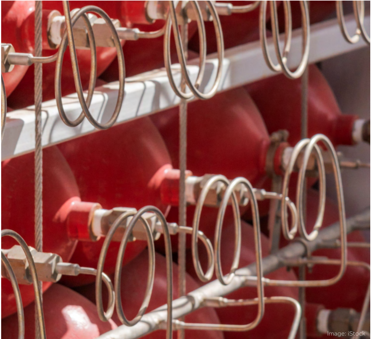
Gaseous hydrogen tube trailers use high-pressure steel or composite cylinders to store and transport hydrogen.
